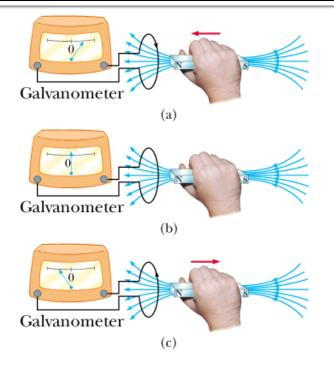
A current flows through the loop when a magnet is moved near it, without any batteries!
