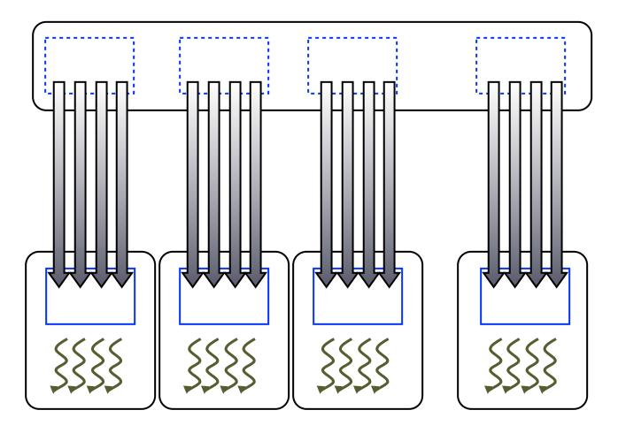
• Loading the subset from global memory to shared memory, using multiple threads to exploit memory-level parallelism.
