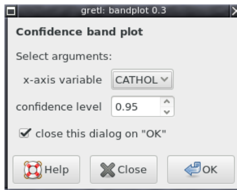
Figure 3.8: Call to bandplot , with special parameter-list inflections. Note the spin-button selector for conf (scalar) and the drop-down selector for xvar (int) as described in the text.
