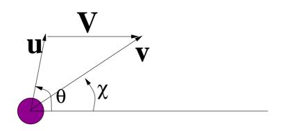
1. The figure above shows a scattered particle (mass  $m_1$ ) with velocity  $\mathbf{v_{1f}}$  and angle  $\chi_1$  as measured in the lab frame and velocity  $\mathbf{u_{1f}}$  and angle  $\theta_1$  as measured in the center of mass frame with  $\mathbf{V}$  denoting the velocity of the center of mass. Assuming that the collision of particle  $m_1$  with the initially stationary particle  $m_2$  is elastic, show that
