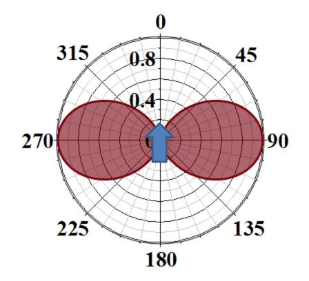
Blue arrow indicates the particle acceleration direction
