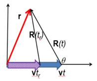
The analysis depends on the ratio of the speed of the particle v to the speed  $c_n$  of electromagnetic waves with the medium --  $\beta_n$ . We showed the following relationship between the lengths R(t),  $R(t_r)$ , and the angle  $\theta$  with the x axis.
